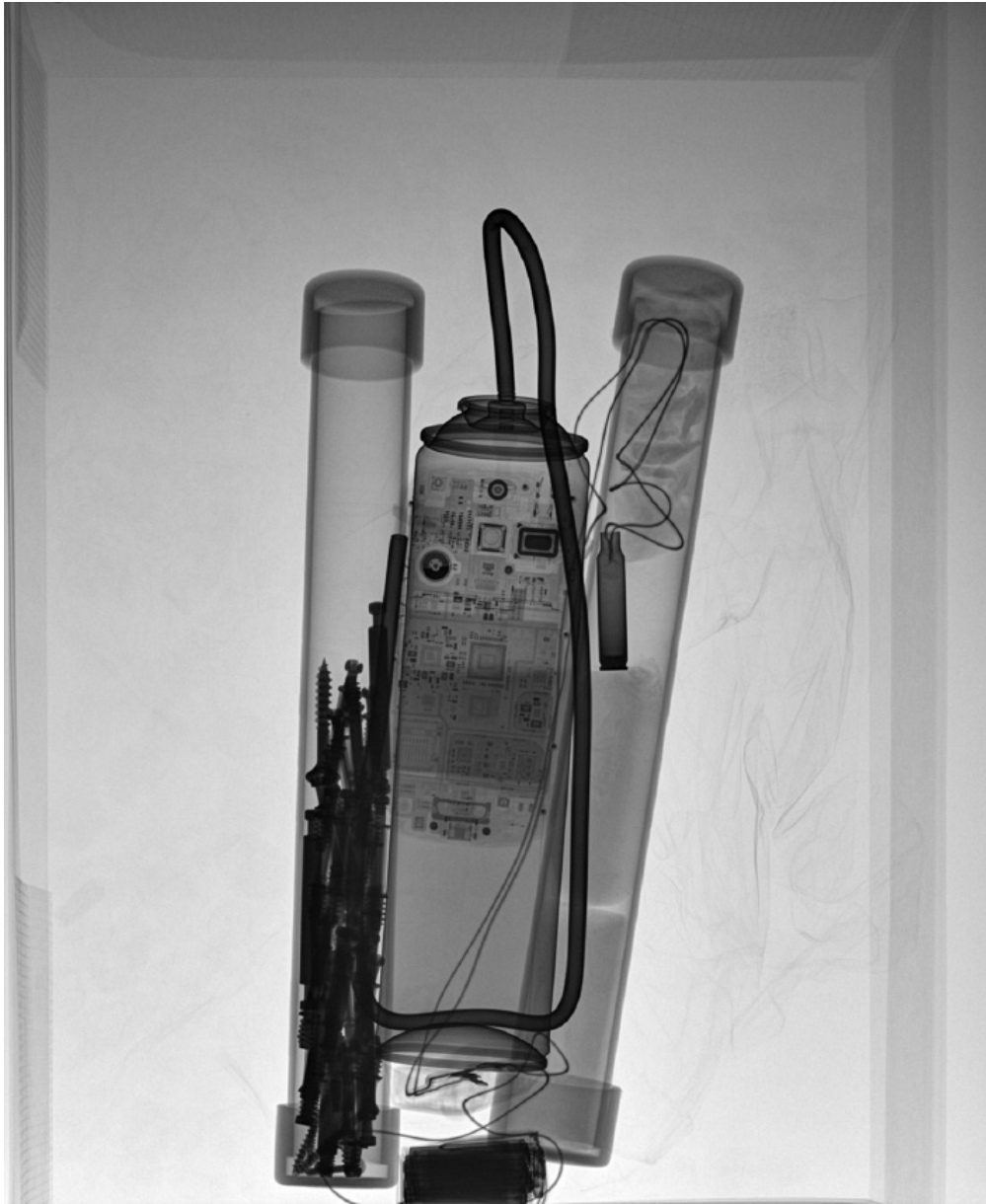
Sample image taken with XRS-3 (15 pulses) on STENÓS panel from 1 meter.
